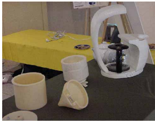
Figure 15 Prototypes of the components of the coffee maker from various materials
